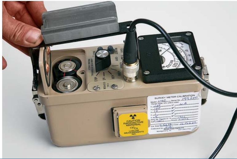
Figure S6.9 Inserting batteries. Note the radiation testing source on the side of the device.
