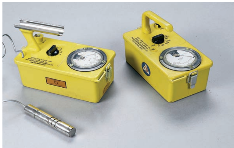
Figure S6.8 Low-range Geiger-Muller-type beta-gamma detector with hotdog probe.
