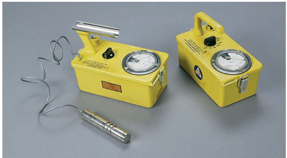
Figure 5.9 Civil Defense radiation detection instruments with “hotdog” probe.
