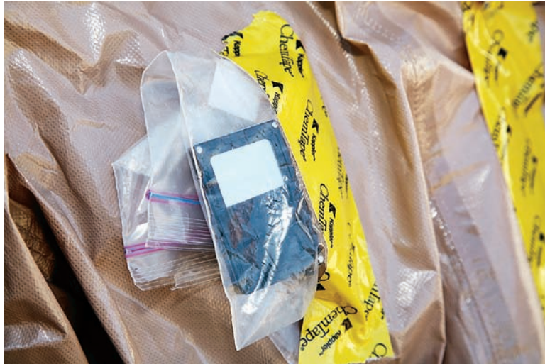
Figure S6.6 Attach the bag containing the TLD to you PPE. You may put the pencil dosimeter and the TLD in the same bag.
