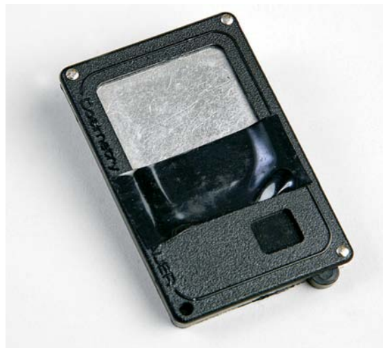
Figure S6.5 Example of a thermoluminescent dosimeter (TLD).
