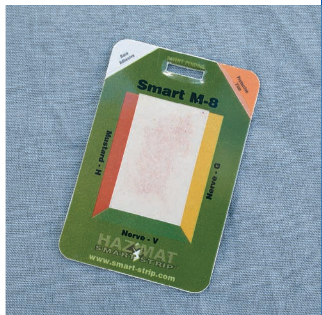
Figure S5.7 Example of a Colorimetric Qualitative Gas Sensor badge.
