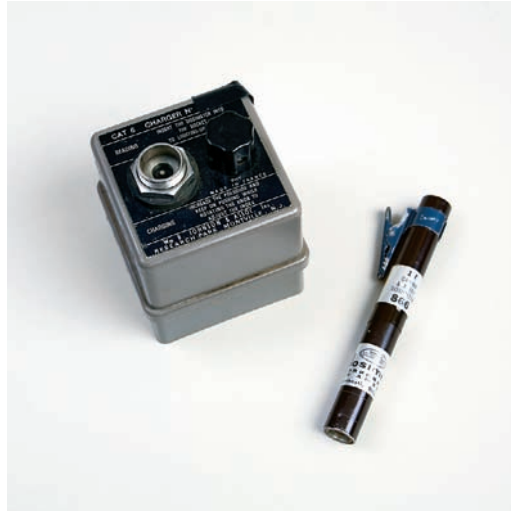
Figure S6.1 Example of a pencil ion chamber dosimeter and charger (calibrator).
