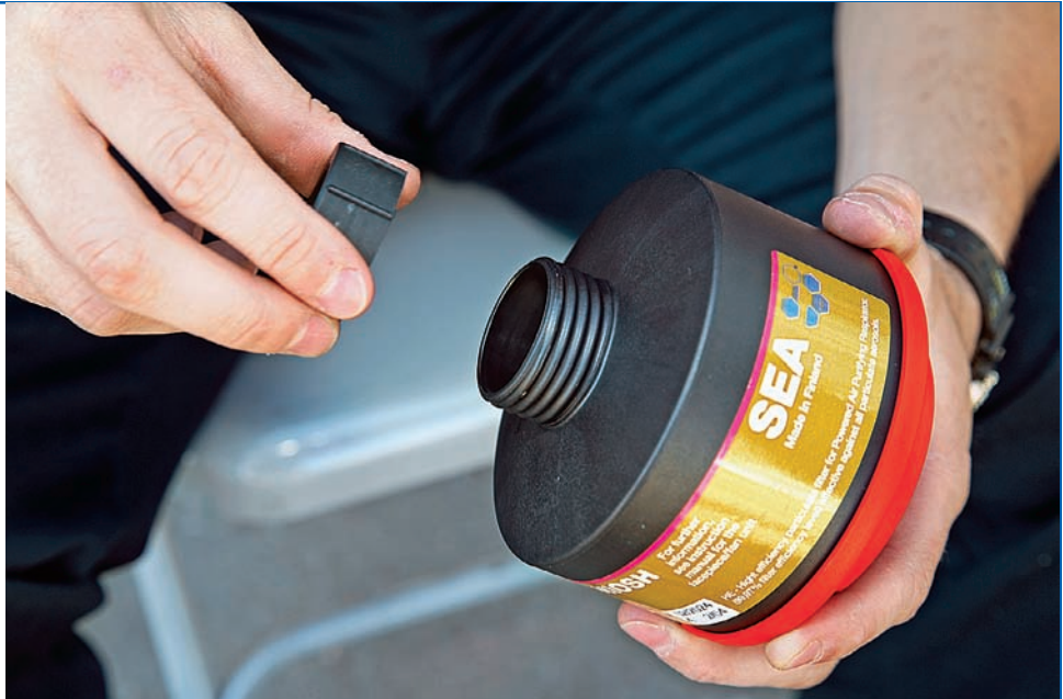
Figure S1.8 Remove filter seals, this is critical!
