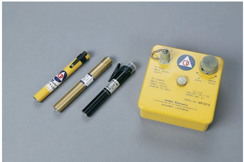
Figure 5.12 Pencil dosimeters and calibrating device.
