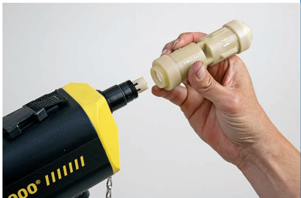
Figure S5.6 PID being tested with check source.
