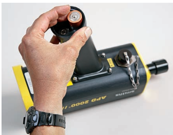
Figure S5.3 Placing batteries into the battery case.
