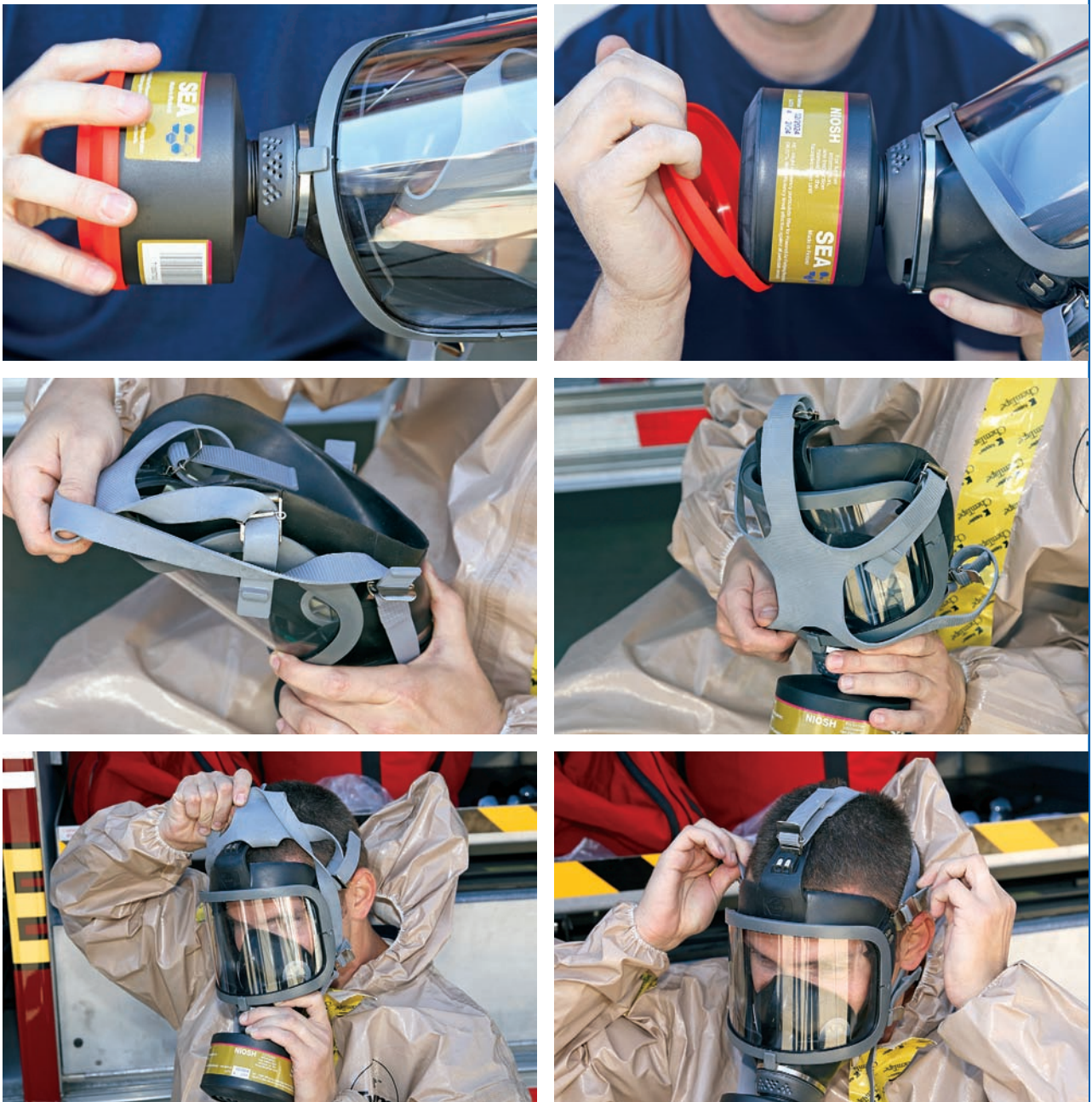
Figure S1.12 Steps for putting on the APR mask.
