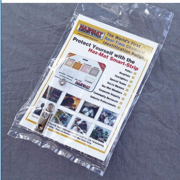
Figure S5.7 Example of a Colorimetric Qualitative Gas Sensor badge.
