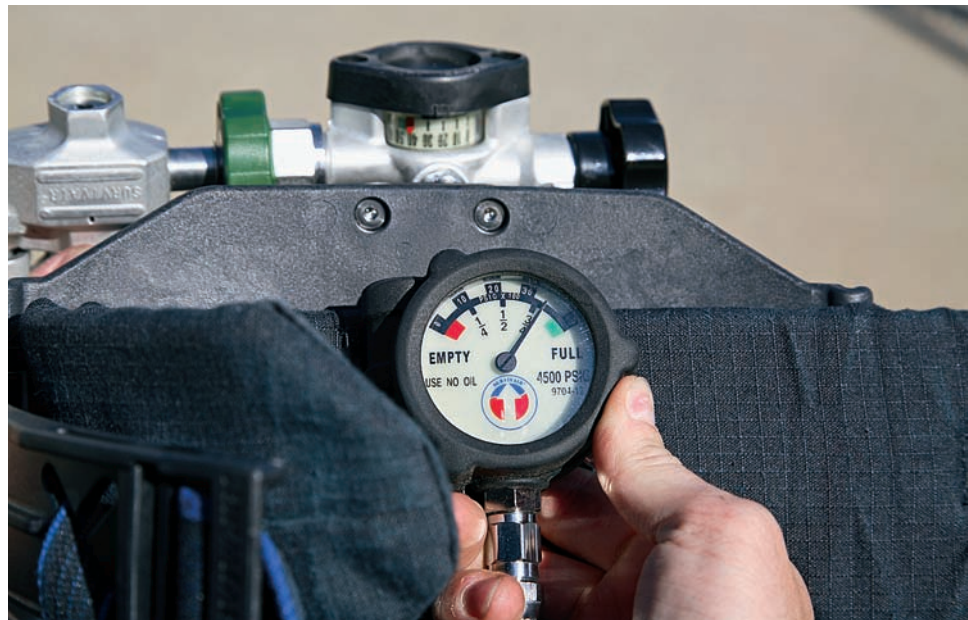
Figure A.9 Compare regulator gauge and tank gauge to confirm they read the same.
