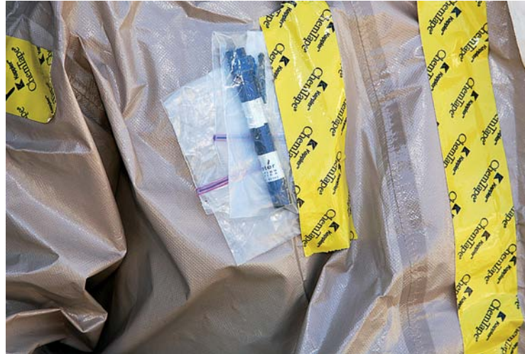
Figure S6.4 Dosimeter in plastic bag attached to PPE.
