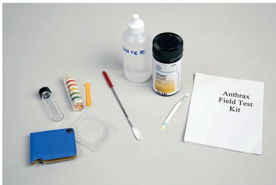
Figure S4.3 Components of a homemade anthrax test kit. Note the white powder on the tip of the spatula.
