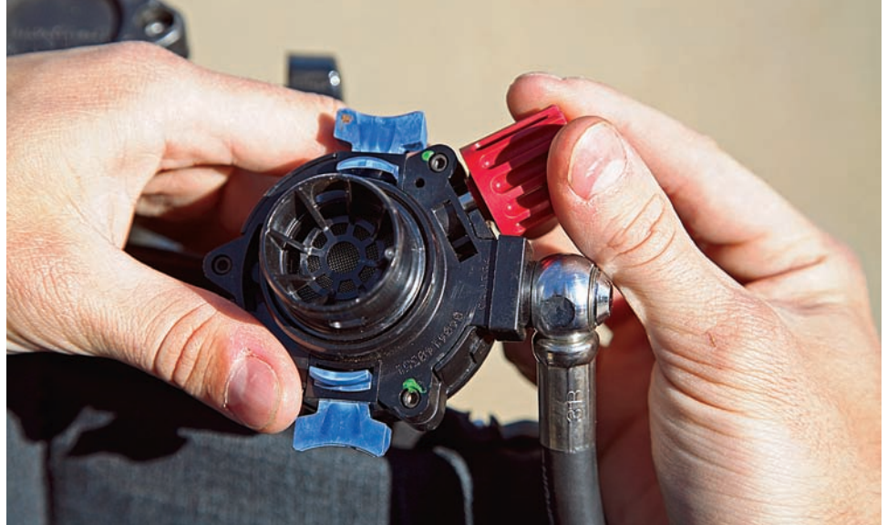
Figure A.10 Activate emergency bypass valve to confirm that you have emergency air flow.
