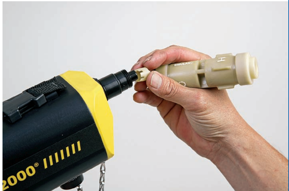
Figure S5.5 Confirm that the air-sample pump is active and the air-sample inlet is not blocked.
